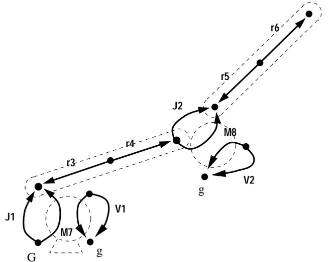
Figure 2. Linear Graph of Two-Link robot
