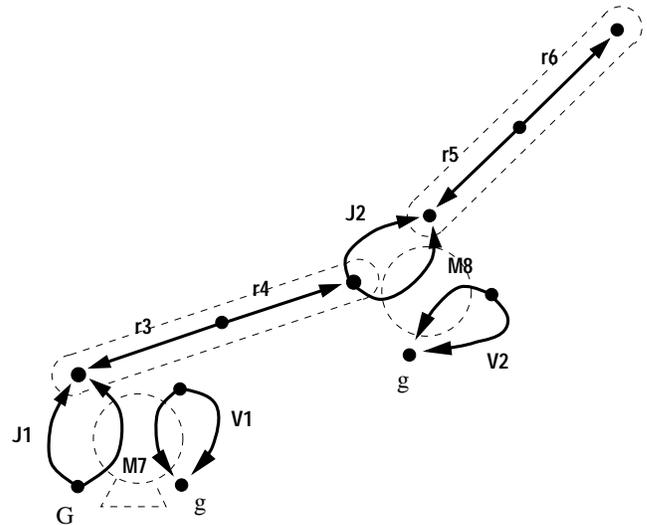
Figure 2. Linear Graph of Two-Link robot
