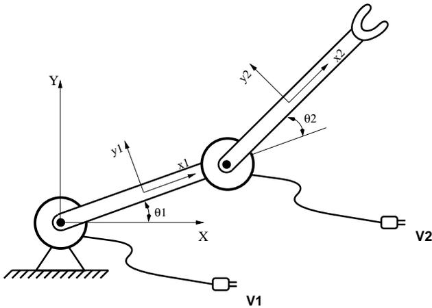
Figure 1. Two-Link Robot Driven by DC Motors
