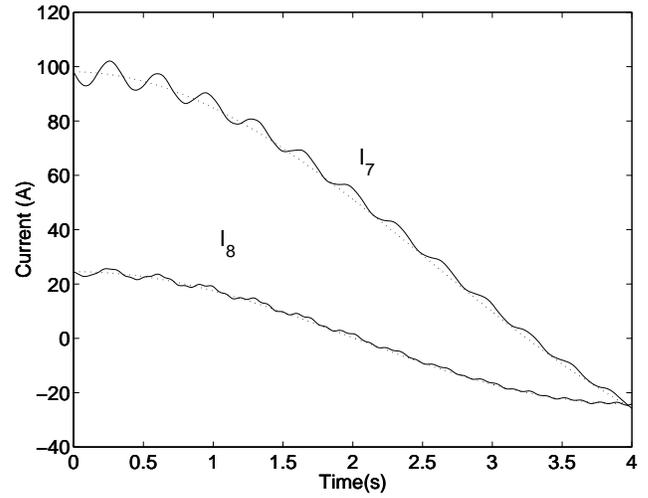
Figure 3. Motor Currents Required for Given Joint Trajectories
