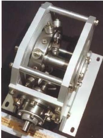
Figure 3: A prototype of spherical Speed-o-Cam
