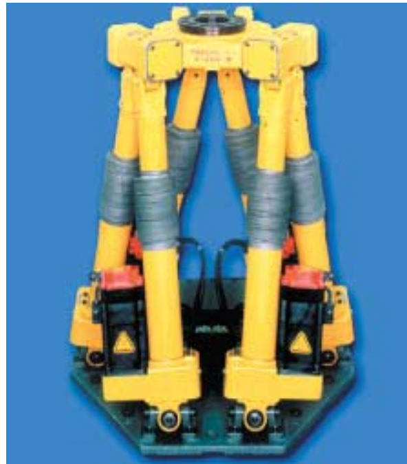
Figure 1: A 6-DOF parallel robot (F-200i) from FANUC Robotics Inc.
