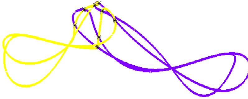
Figure 7: Intersection curves C_{12} and C_{13} with the intersection points denoted * of the two curves in 3D Cartesian space for the Y Star TPM (8 real solutions)
