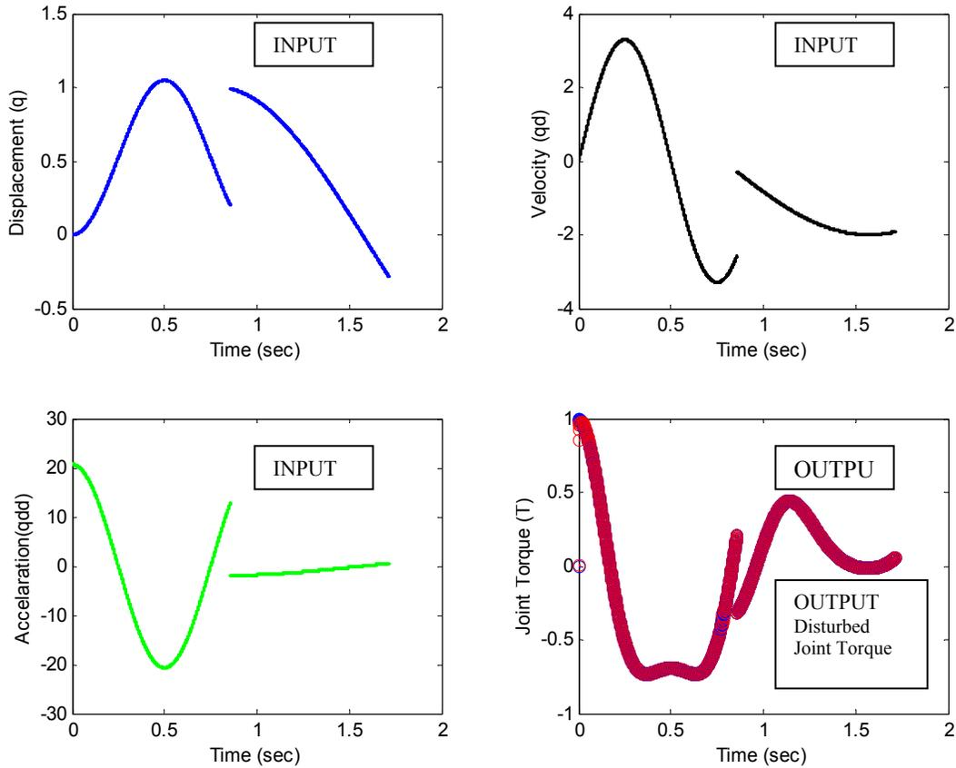
Figure 5 First joint inputs and torque approximation of robot by NN with disturbance.
