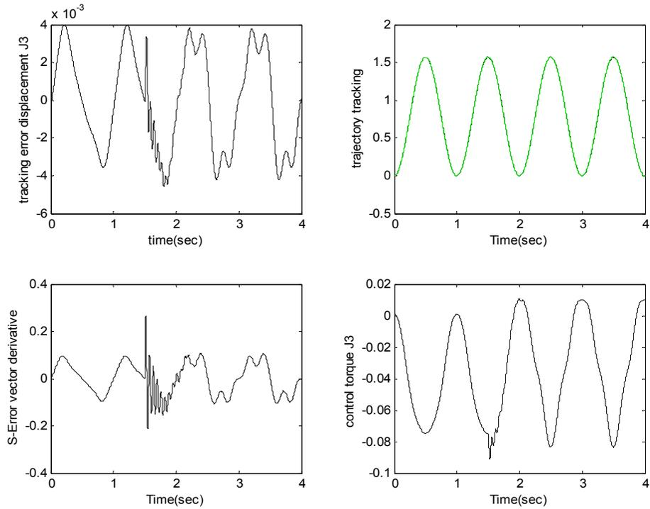
Figure 9 Simulation results for joint three of Phantom robot.
