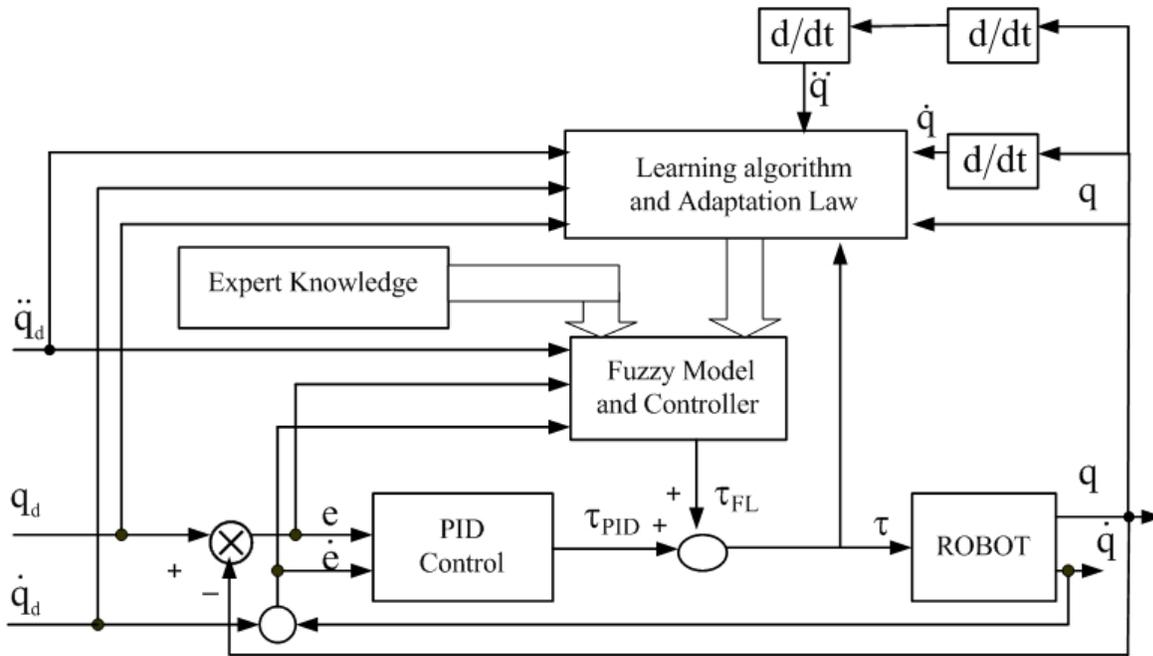
Figure 1 Proposed controller block diagram.
