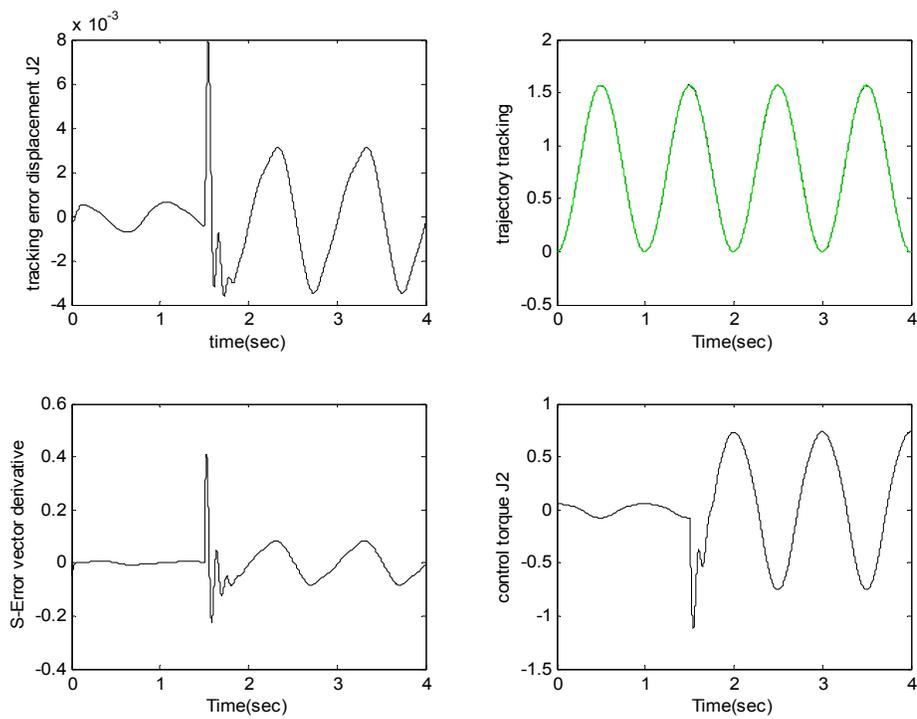
Figure 8 Simulation results for joint two of Phantom robot.
