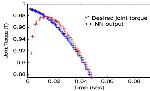
Figure 4 Joint torque approximation for the first 0.1 second of robot by NN.
