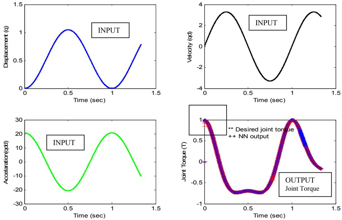
Figure 3 First joint inputs and torque approximation of a two-link serial robot by NN.
