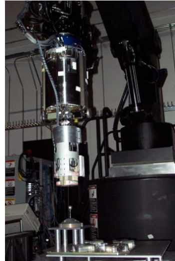
Figure 1: MDR end-effector mounted on STVF test bed
