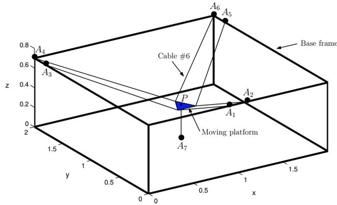
Figure 2: A 6-DOF parallel mechanism driven by seven cables for its reference orientation.
