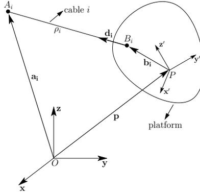
Figure 1: Kinematic modeling.
