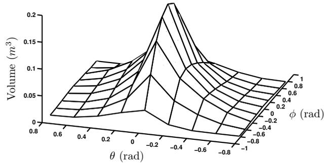
Figure 5: Volume of the COWCW for different orientations of the mobile platform of the mechanism shown in Figure 2, with  $\psi = 0$ .
