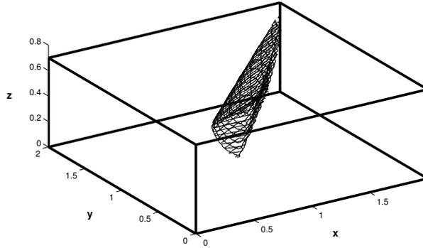
Figure 4: The COWCW of the mechanism shown in Figure 2 for  $\phi = -\pi/12$ ,  $\theta = -\pi/12$  and  $\psi = 0$ .
