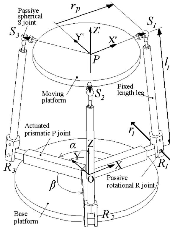
Figure 1: The 3-PRS parallel manipulator - Mechanism architecture and vector model from Carretero et al. [14]
