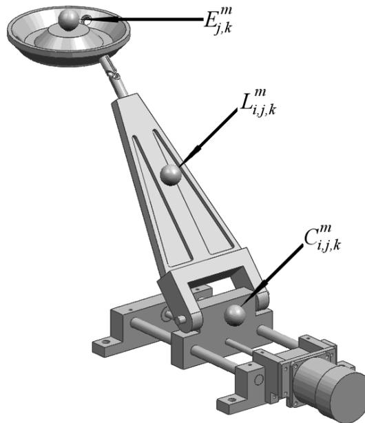
Figure 3: One leg of the 3-PRS manipulator - Arbitrary location of markers for calibration method.
