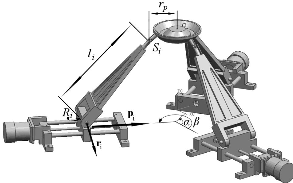
Figure 2: The 3-PRS parallel manipulator - CAD representation of physical construction.
