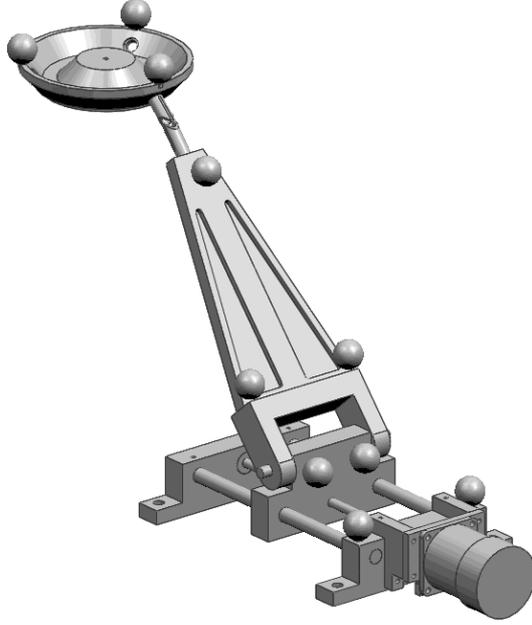
Figure 4: One leg of the 3-PRS manipulator - Location of virtual markers for preliminary testing.
