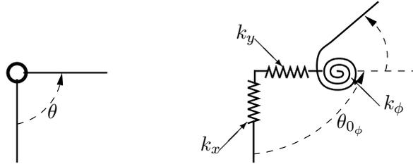
Figure 1: Conventional and realistic compliant revolute joint models
