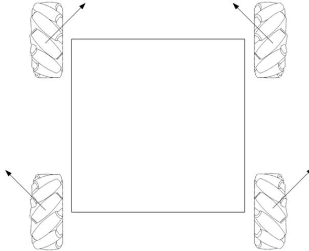
Figure 5: Mecanum Wheel Orientation on the OmniMaxbot (Top View)
