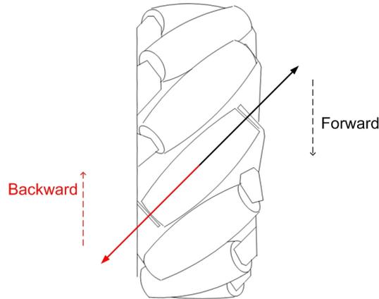
Figure 3: Forces on a Mecanum Wheel (Bottom View)
