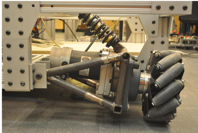
Figure 6: Suspension System
