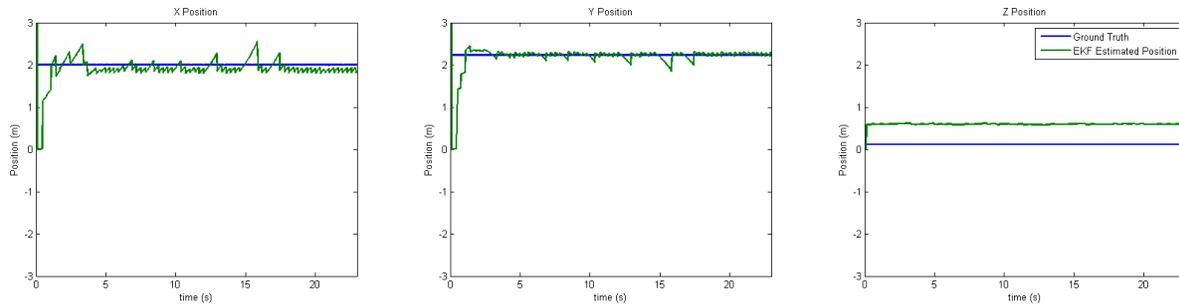
Fig. 6. Static quadrotor EKF Estimation vs. Ground Truth
