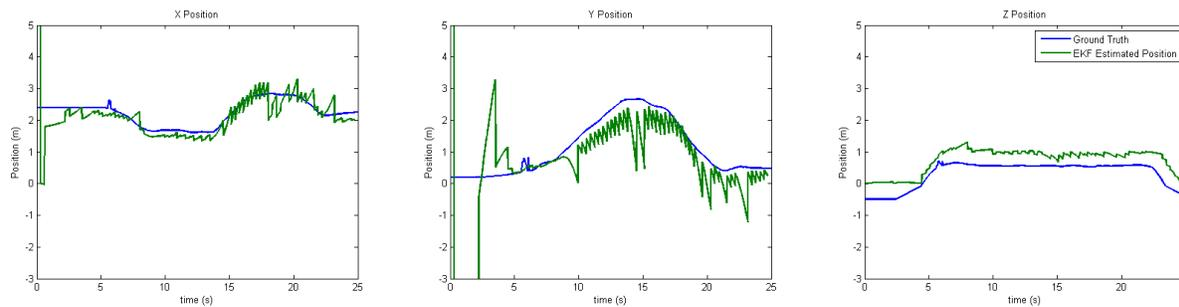
Fig. 7. Moving quadrotor EKF Estimation vs. Ground Truth
