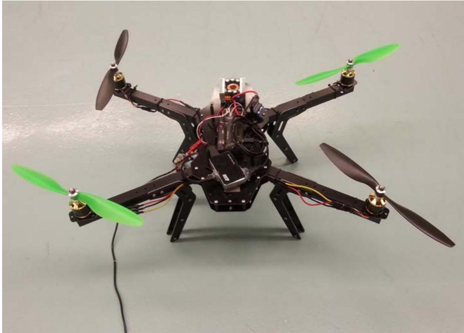
Fig. 2. The quad-rotor chassis for UAV platform
