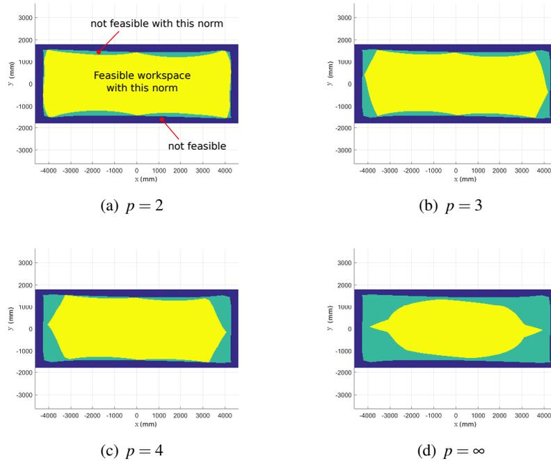
Fig. 4. Achievable zero rotation static workspaces using different unconstrained  $p$ -norm optimization algorithms at  $z = 1250$  mm showing the wrench-closure and wrench-feasible workspaces (WCW and WFW respectively).
