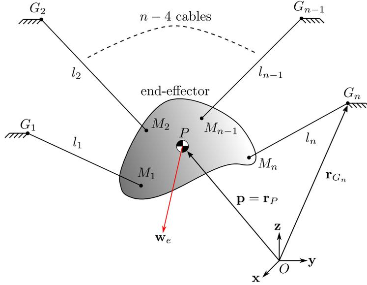
Fig. 1. Spatial cable robot kinematic model.
