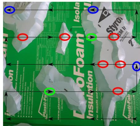
Fig. 2. Trajectory Overlaid on Mock-Up Mine Surface (Via Points Used for Angle Shown in Green, Distance in Blue, and Missing Points in Red)
