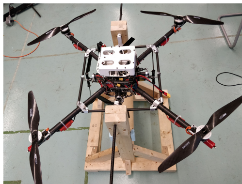
Fig. 6. The OmniRaptor on the Test Stand
