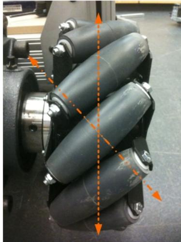
Figure 2: Motion of a Mecanum Wheel
