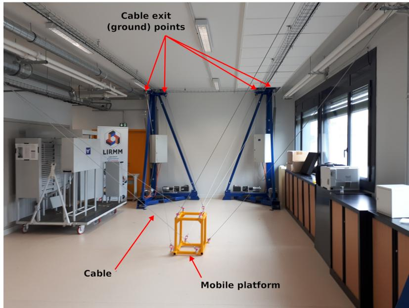
Fig. 2. The suspended cable robot considered in this work.
