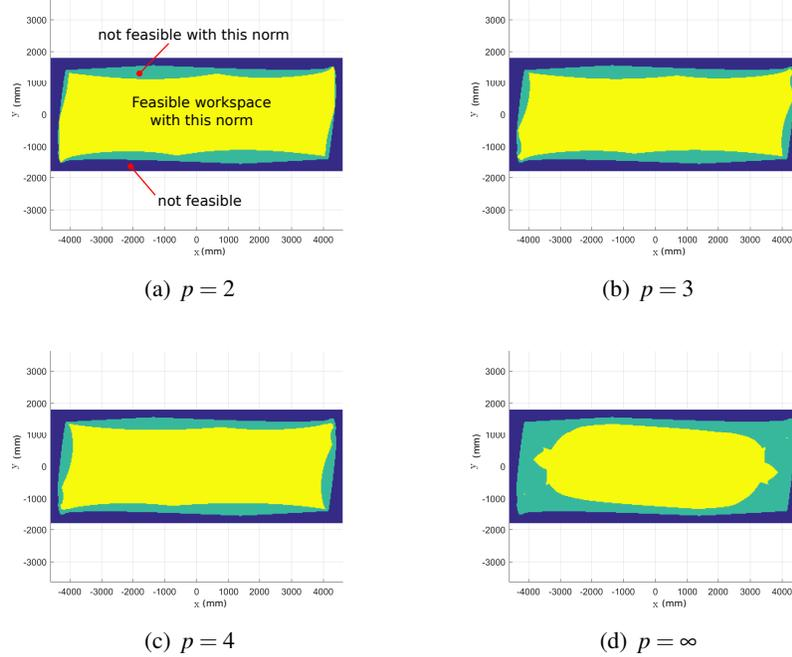
Fig. 5. Achievable zero rotation static workspaces using different unconstrained  $p$ -norm optimization algorithms at  $z = 2250$  mm showing the wrench-closure and wrench-feasible workspaces (WCW and WFW respectively).
