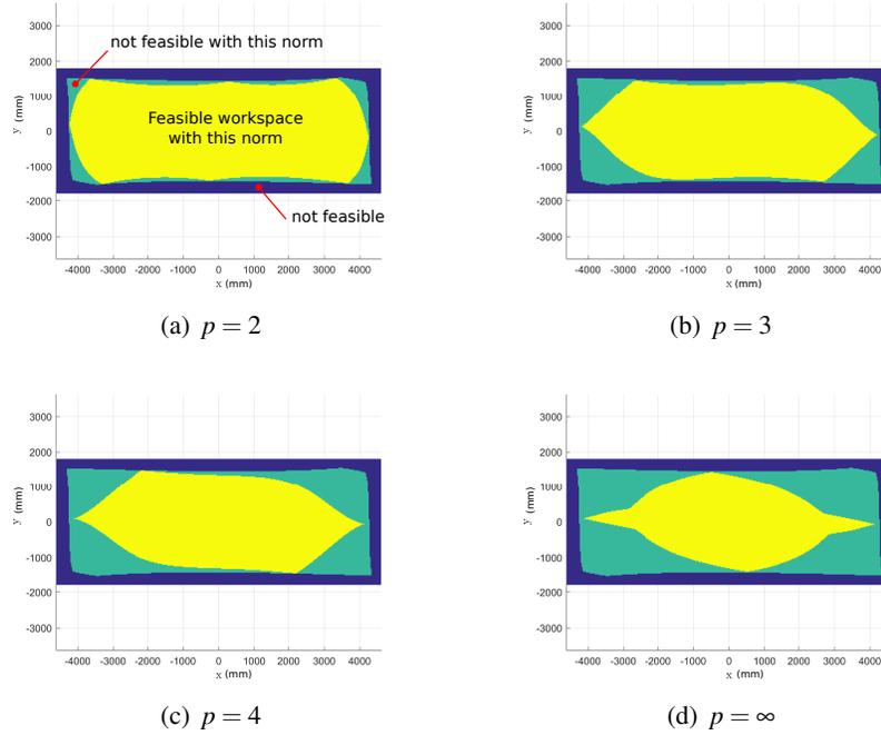
Fig. 3. Achievable zero rotation static workspaces using different unconstrained  $p$ -norm optimization algorithms at  $z = 250$  mm showing the wrench-closure and wrench-feasible workspaces (WCW and WFW respectively).
